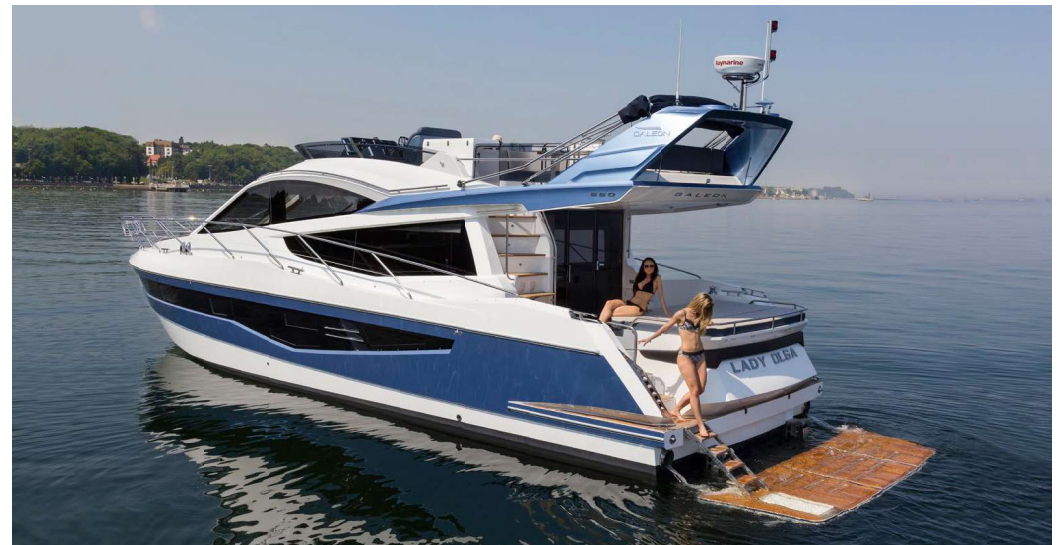
A hydraulic bath platform lowers into the water —
